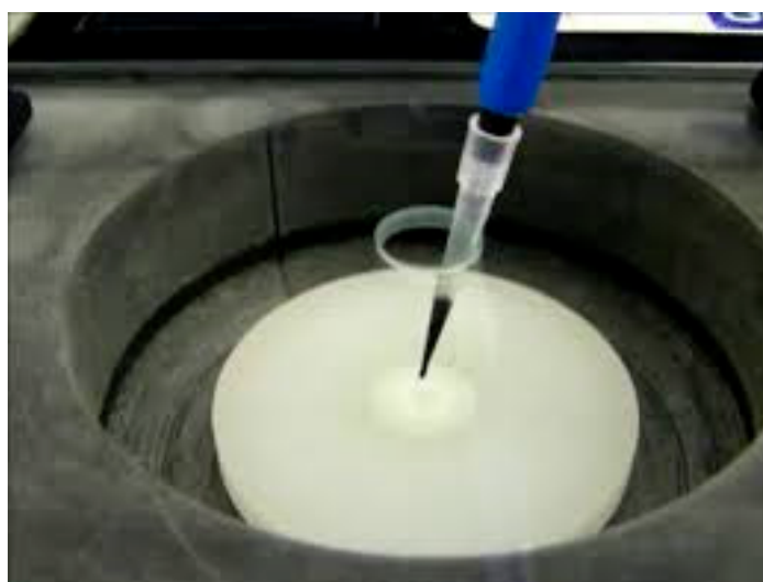
Figure 1. Spin-coating process (feeding of dissolved metal solution onto ITO substrate using micropipette).
