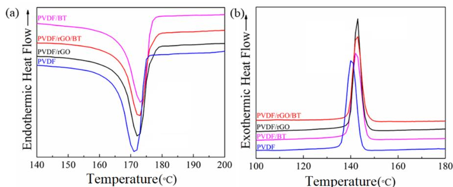
**Figure 3.** DSC second melting (a) and cooling (b) curve of PVDF, PVDF/BT, PVDF/rGO, and PVDF/rGO/BT nanocomposite fibers.
