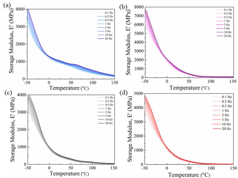
**Figure 4.** Storage modulus vs. temperature for (a) PVDF, (b) PVDF/BT, (c) PVDF/rGO, and (d) PVDF/rGO/BT fibers obtained from DMA measurement. In all cases, the storage modulus was determined at a range of oscillation frequencies, as indicated.
