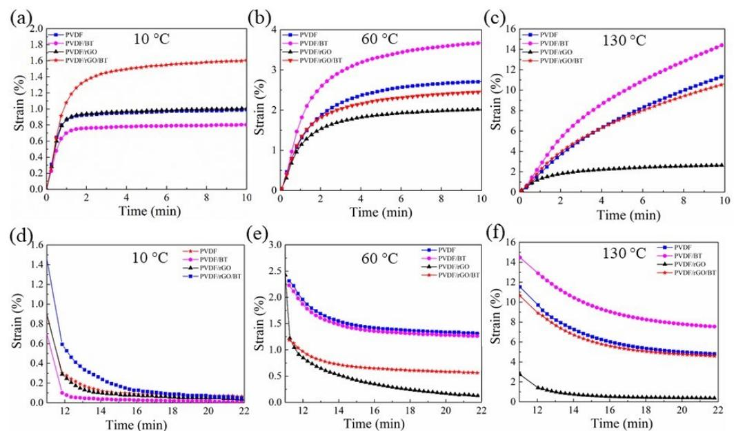
**Figure 7.** The creep behaviours (a–c) and creep recovery (d–f) of the melt-spun PVDF, PVDF/BT, PVDF/rGO, and PVDF/rGO/BT fibers at temperature (10, 60, 130 °C).
