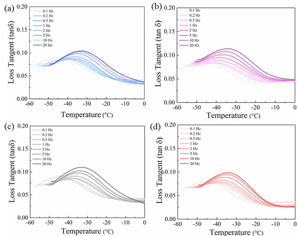
**Figure 5.** Temperature and frequency dependence of  $\tan \delta$  for (a) PVDF, (b) PVDF/BT, (c) PVDF/rGO, and (d) PVDF/rGO/BT nanofibers.
