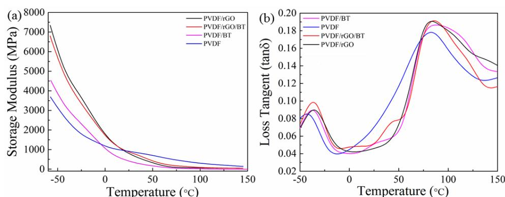
**Figure 6.** Dynamic mechanical analysis of the PVDF nanocomposite fibers at frequency 1 Hz: (a) storage modulus, (b) loss tangent ( $\tan \delta$ ).
