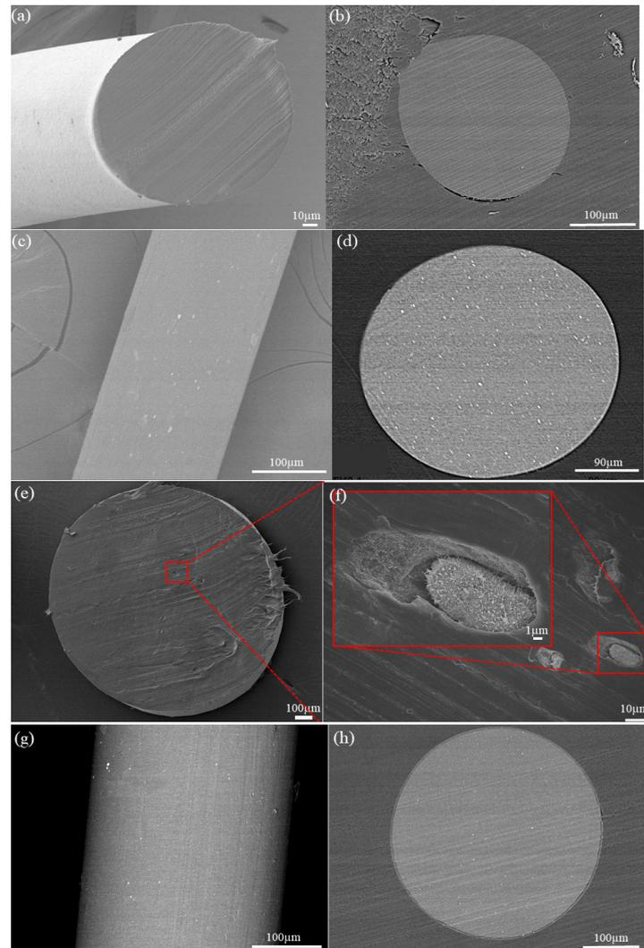
**Figure 2.** SEM images of the nanocomposite fibers: (a) surface and (b) cross section of PVDF fiber; (c) surface and (d) cross section of PVDF/BT (10 wt%); (e,f) low and higher magnification of cross-section of PVDF/rGO fiber (0.5 wt%) with the low content of graphene nanosheets with the dimension of 200–400 nm; and (g,h) surface and cross section of PVDF/rGO/BT fiber.
