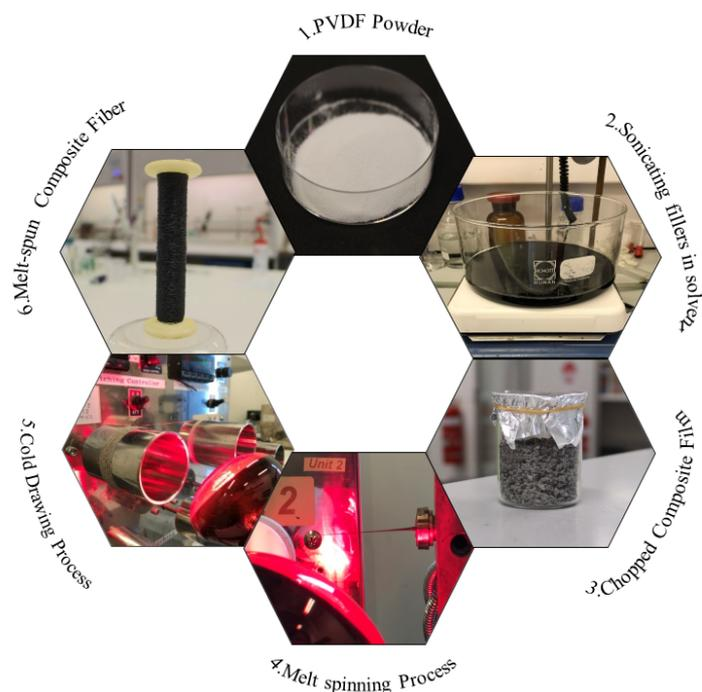
**Figure 1.** Preparation process of PVDF/rGO nanocomposite fibers.
