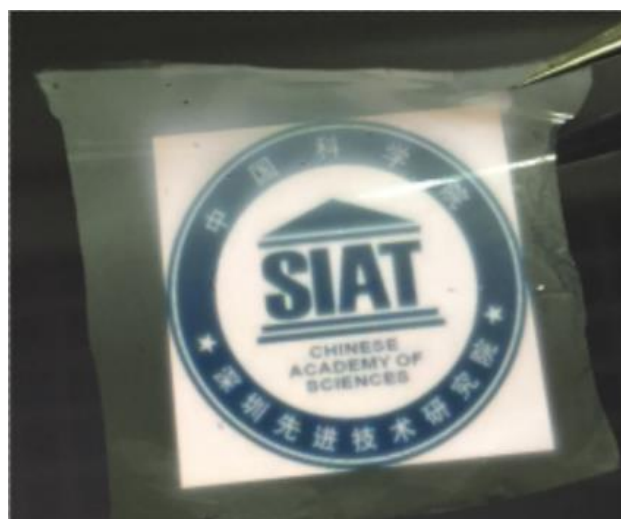
Figure S4. The optical photo of single-layered PE/BNNPs film.
