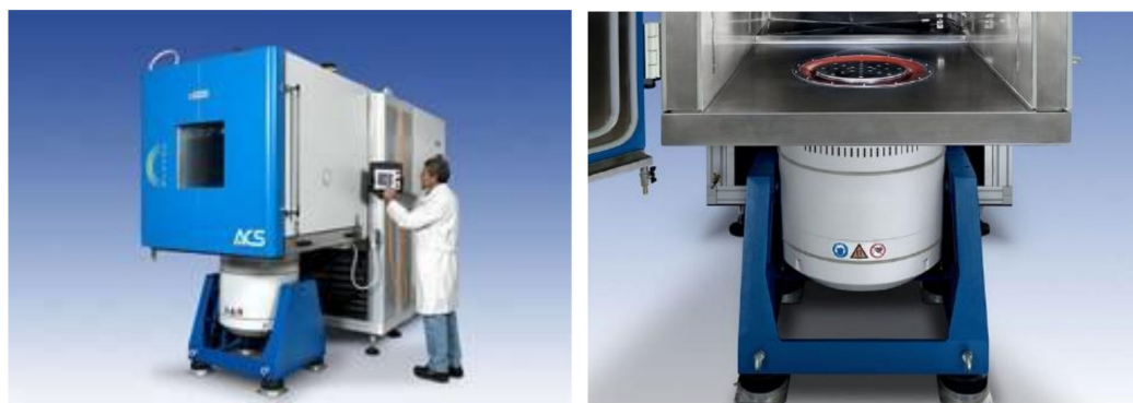
Figure 2. Angelantoni CH250 climatic chamber + TIRA S55240/LS—Vibration system.
