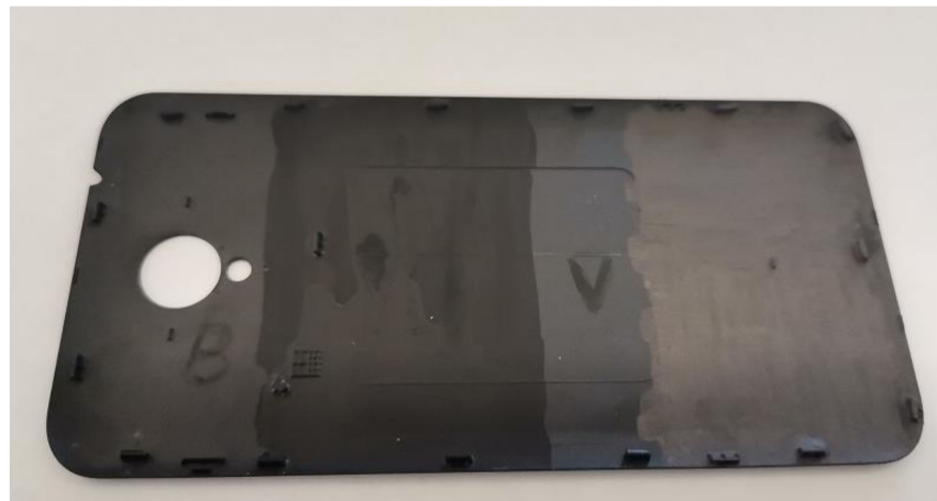
Figure 12. Cellular phone back side chassis coated with 2 paints samples.
