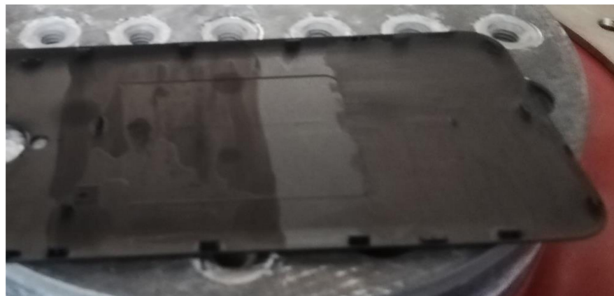
Figure 13. The sample coatings after two combined cycles of temperatures from +60\text{ }^{\circ}\text{C} to -20\text{ }^{\circ}\text{C} and relative humidity from RH 90% to 10% with 8 h maintaining time at higher and lower temperatures.
