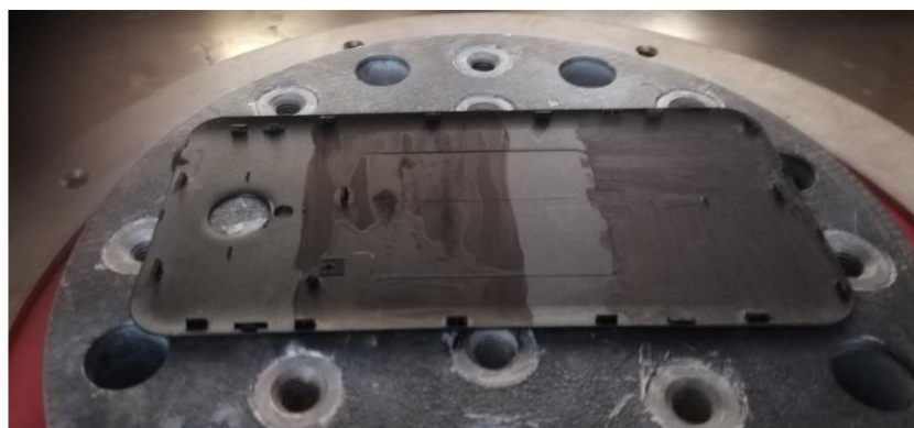
Figure 16. The sample coatings after vibrations.
