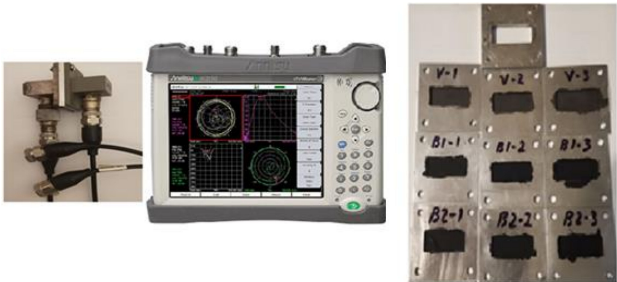
Figure 1. The measuring setup for EMI-shielding efficiency based on the ANRITSU Vector Network Analyzer.
