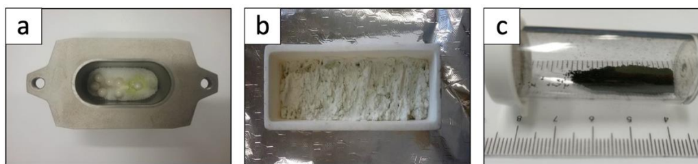
Figure 1. (a) Tungsten carbide container including sample mixture and ZrO 2 balls; (b) ball-milled mixture collected in alumina boat; (c) WS 2 nanosheets obtained after CVD reaction.
