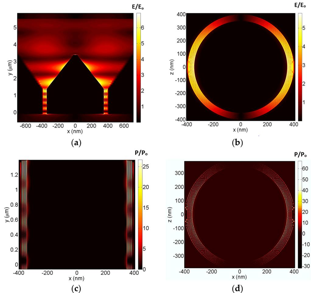
**Figure 2.** The three-dimensional finite-difference time-domain of normalized electric fields ( $E/E_0$ ) and absorption ratios ( $P/P_0$ ) at a wavelength of 1476 nm. (a) An XY vertical cross-section of the graphene metamaterial embedded Bundt optenna, (b,d) An XZ horizontal cross-section at the waveguide input, and (c) an XY vertical cross section of the waveguide.
