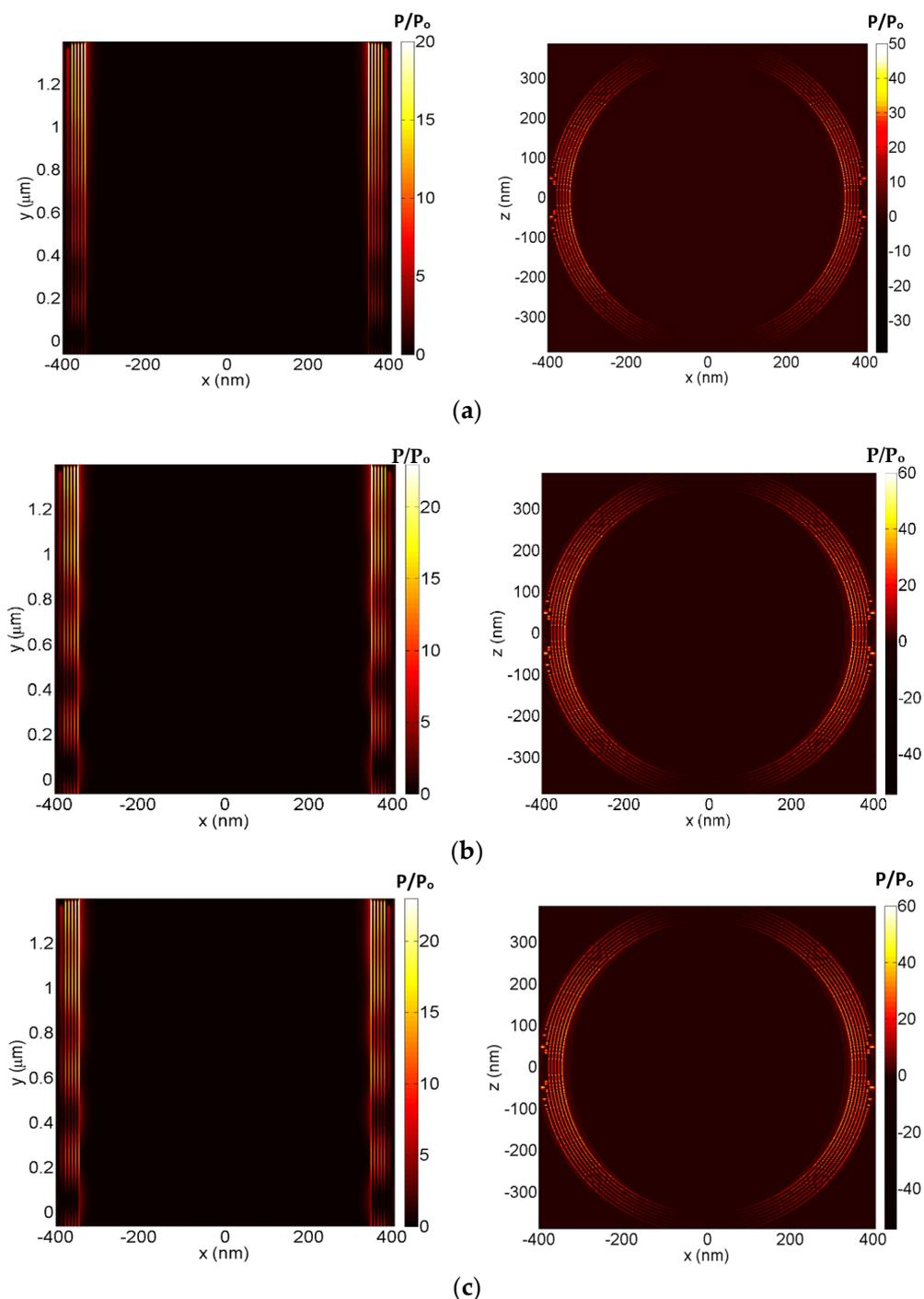
**Figure 3.** The three-dimensional finite-difference time-domain of the absorption ratios ( $P/P_0$ ) for the XY cross section and XZ cross section inside the plasmonic waveguide at some selected wavelengths: (a) 1300 nm, (b) 1600 nm, (c) 1439 nm.
