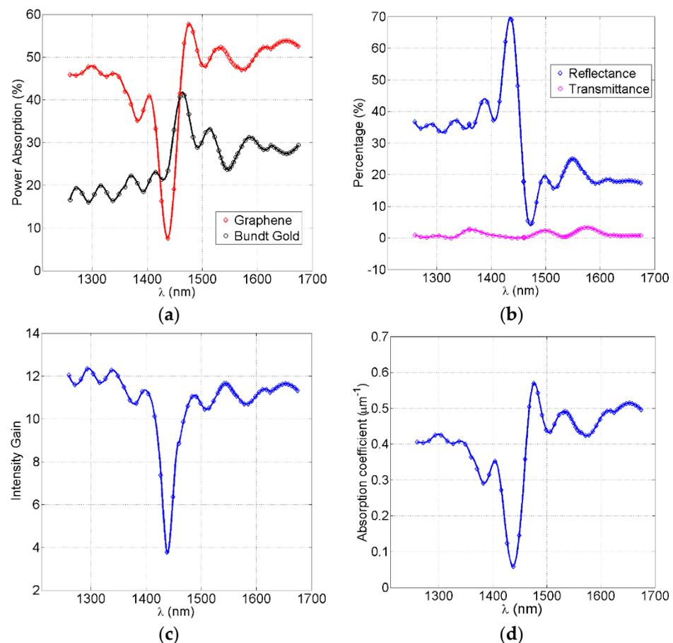
**Figure 4.** The performance evaluation of the graphene metamaterial embedded Bundt optenna device. (a) The percentage of incident power absorption in the graphene metamaterial and device gold surfaces. (b) The percentage of incident power reflected at the device input and transmitted at the device output. (c) The gain (i.e., enhancement) in infrared intensity at the output of the first–stage horn. (d) The absorption coefficient of the graphene metamaterial per micrometer length.
