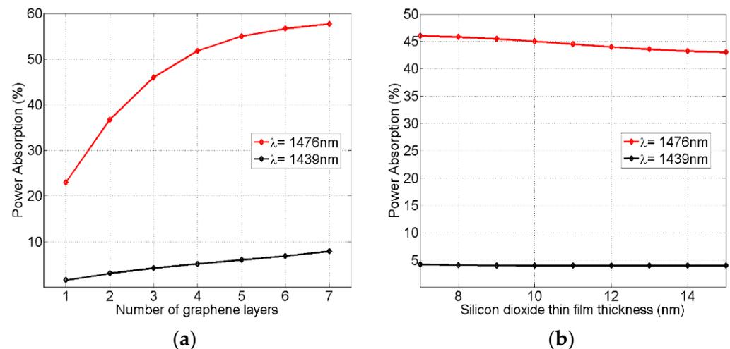
**Figure 6.** The variations in the metamaterial absorbed power ratio as a function of the number of concentric graphene layers (a), and the thickness of silicon dioxide ( $\text{SiO}_2$ ) thin films (b). The selected wavelengths of 1476 nm and 1439 nm corresponded to the maximum and minimum graphene absorption ratios in Figure 4a, respectively.
