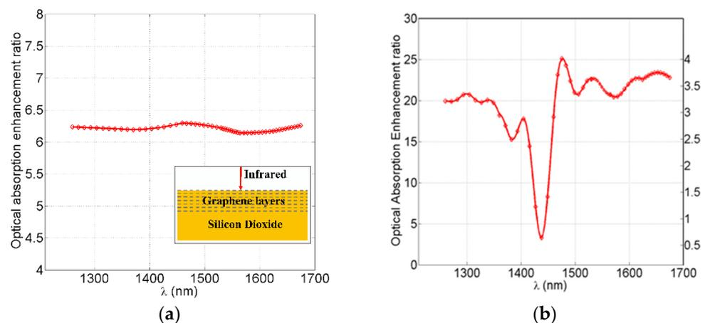
**Figure 5.** The optical absorption enhancement performance for different cases: (a) standalone graphene metamaterial (seven layers) with a perpendicular infrared incidence, as shown in the inset. The absorption was compared to standard standalone monolayer graphene, (b) graphene metamaterial Bundt optenna compared to the standalone metamaterial in case 'a' on the right axis, and compared to the standard standalone monolayer graphene on the left axis.
