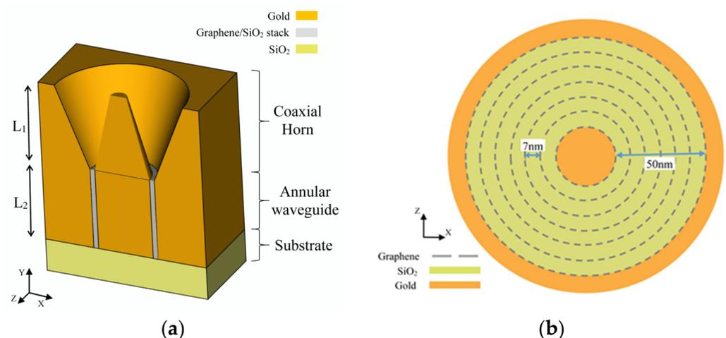
**Figure 1.** The graphene metamaterial embedded Bundt optenna device configuration. (a) A three-dimensional schematic diagram of the device with an XY cross section showing different stages. (b) A magnified XZ cross section in the waveguide with a cylindrical graphene metamaterial stack showing the alternating and concentric silicon dioxide thin films and graphene layers.
