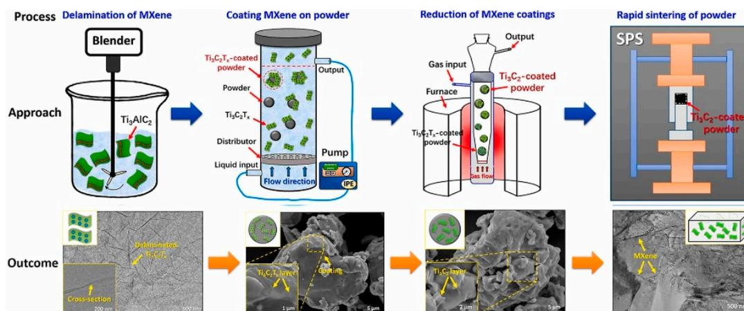
**Figure 7.** Schematic illustration of the powder metallurgy process. Reprinted with permission from Ref. [54]. 2020, Elsevier.
