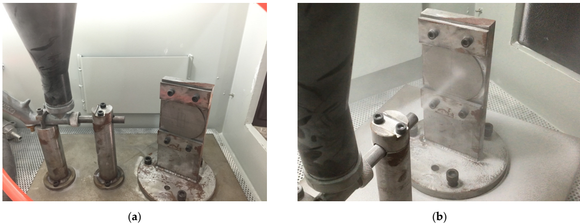
Figure 4. Photographs of the assembled erosion test rig. (a) Photo of the blast gun, hopper, and specimen. (b) Photo taken during an erosion test.
