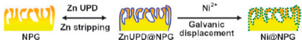
Figure 7. Preparation of a Ni-coated NPG electrode using galvanic replacement of Zn with nickel. Reprinted with permission [140].
