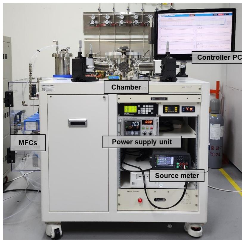
**Figure 6.** (a) Schematic illustration of the experimental setup for measuring the gasochromic-resistive hybrid hydrogen sensor and (b) photograph of the experimental setup.
