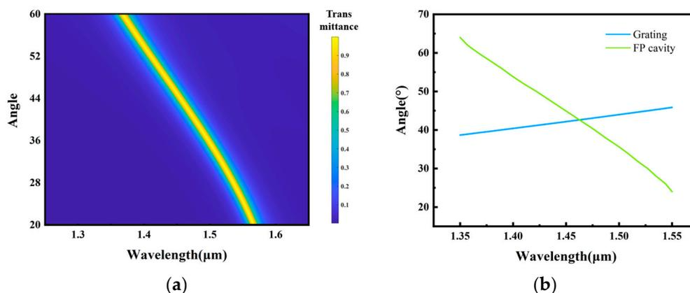
**Figure 3.** (a) FP cavity transmission peak at different incident angles (20 $^\circ$  (1.57  $\mu\text{m}$ ) to 60 $^\circ$  (1.35  $\mu\text{m}$ )). (b) Relationship between the wavelength and the angle for the FP cavity and the metasurface. The intersection indicates that only a single wavelength can pass through the FP cavity.
