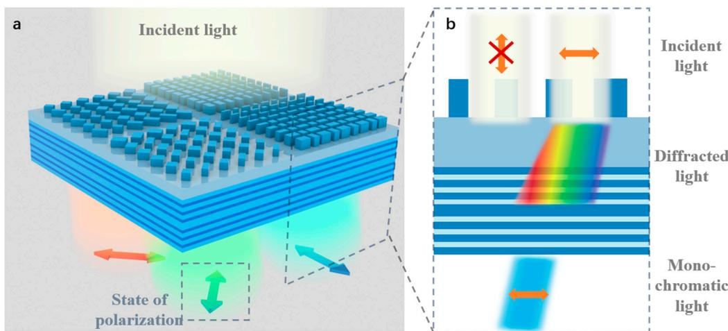
**Figure 1.** (a) Schematic of the proposed polarization spectral detector with multiple mosaic channels. (b) Schematic diagram of light propagation.
