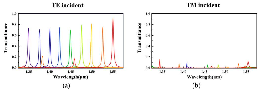
**Figure 4.** Simulation result of the on-chip polarized spectral detector. (a) The transmission spectra of the nine-channel wavelength bands under TE-polarized incident light. (b) The transmission spectra under TM-polarized incident light. The transmission of TM-polarized light is well suppressed.
