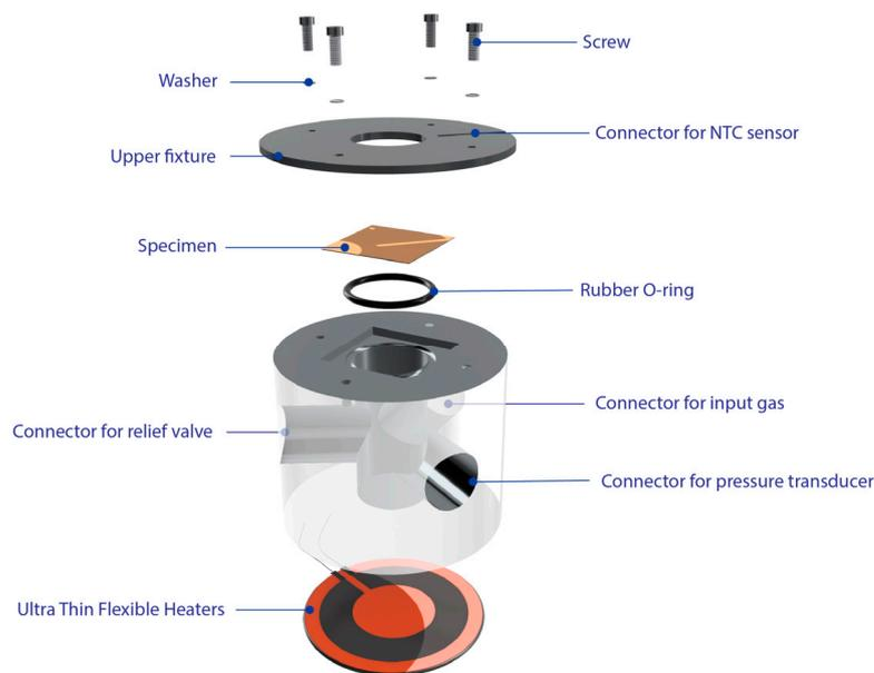
Figure 4. Illustration depicting the chamber setup.
