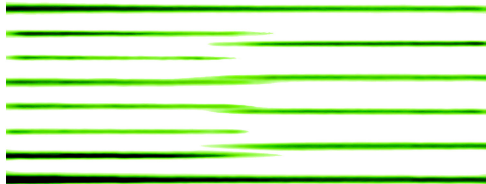
Figure 7. Profile of intensity of diffraction pattern from the germanium layer on Si(111) during the transition from the 7 \times 7 to 5 \times 5 superstructure.
