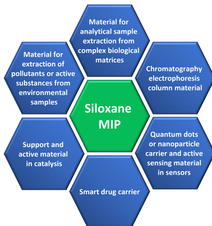
Figure 2. Application areas of siloxane molecularly imprinted polymers.
