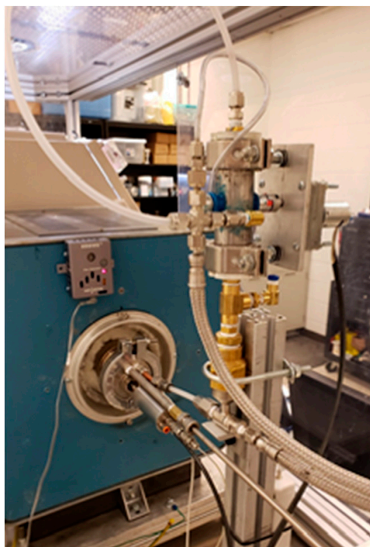
Figure 1. Custom fuel injector and particle injector attached to the inlet of the reactor.
