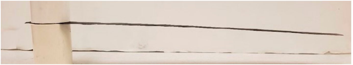
Figure 13. CFRP-CNT strip (cantilevered, with thin polymer binder). The material is lower density than CFRP, more flexible, and is expected to have lower strength in compression than CFRP.
