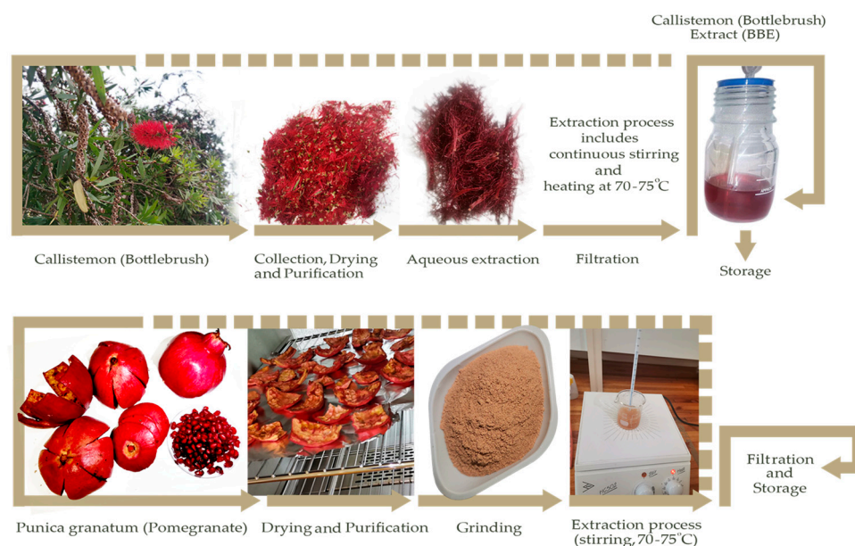
Figure 1. The extraction process of the two selected plants, Callistemon (Bottlebrush) and Punica granatum (pomegranate) peel extracts, respectively.
