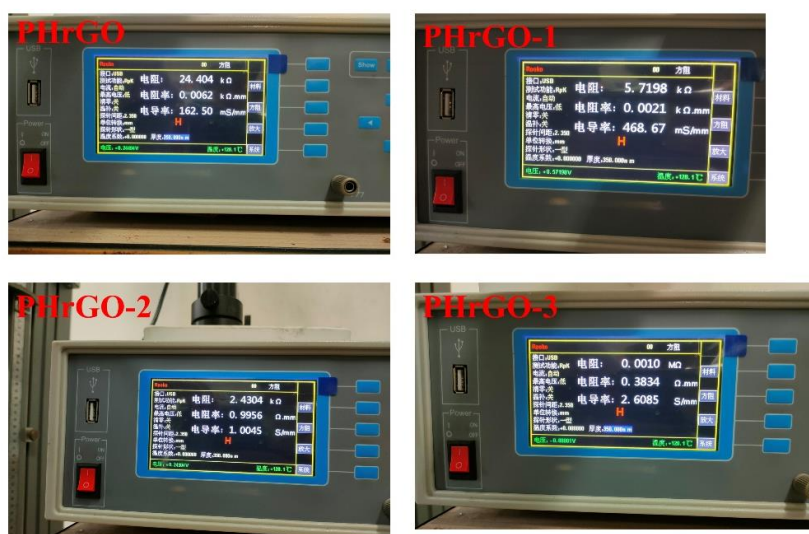
Figure S3. Image of conductivity testing of PHrGO film using a four probe tester
