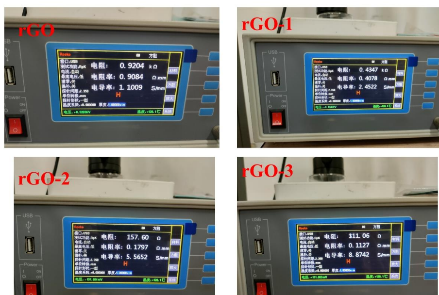
Figure S2. Image of conductivity testing of rGO film using a four probe tester
