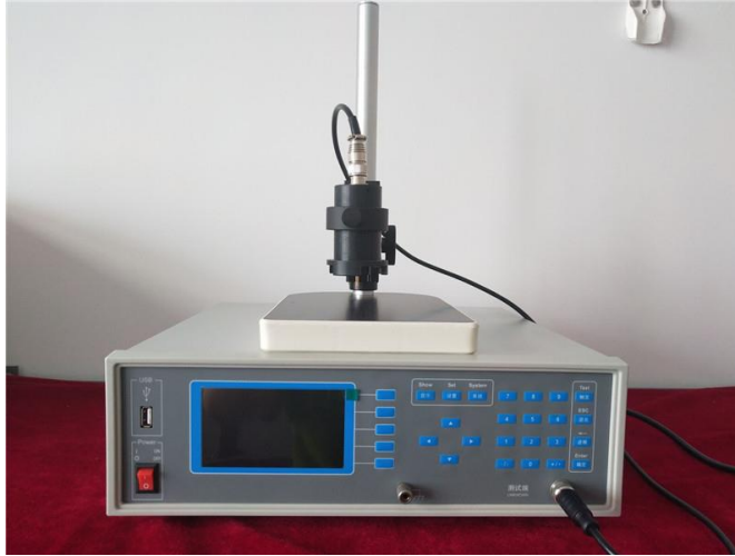
Figure S4. Optical photograph of a multi-function digital four probe tester.
