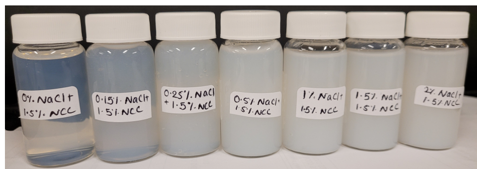
Figure 23. Appearance of 1.5 wt% NCC dispersion samples with the addition of salt (NaCl).
