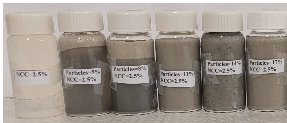
Figure 29. Creaming in suspensions of light hollow spheres at different particle concentrations (wt%) at a fixed NCC concentration of 2.5 wt%. The suspensions were left on the shelf for several months.
