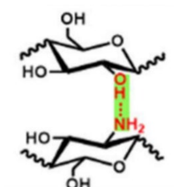
Fig. S6 Hydrogen bonding interaction between the hydroxyl group of CKF and the amino group of CS.
