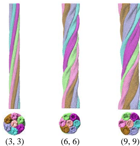
Figure 1. Nanoropes including carbon nanotubes (CNTs) with chiralities (3, 3) (left), (6, 6) (middle), and (9, 9) (right).
