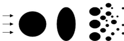
Figure 3. Schematic of droplet secondary breakup.
