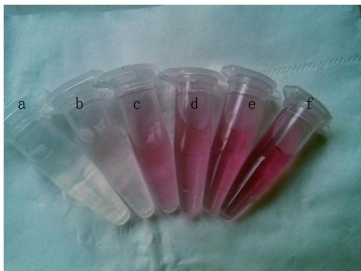
Figure S6 The color change of the AuNP 6 -HAuCl 4 -H 2 O 2 system
