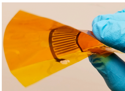
Figure 9. G-CMC filter devices were rolled into a cylinder during mechanical stress tests. There were no measurable differences in frequency response behavior between rolled and unrolled states. As expected, the R and C component values of the individual filters were also unaffected from rolling.
