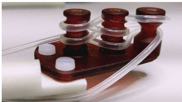
Figure 1. Tube phantom filled with redispersed tracer in water, mounted on the robot arm.
