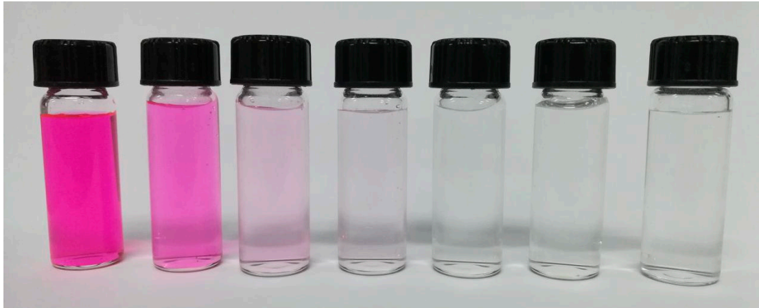
Figure S5. The color change of RhB solution from 0, 10, 20, 30, 40, 50, 60 min under UV-vis light (from left to right) .
