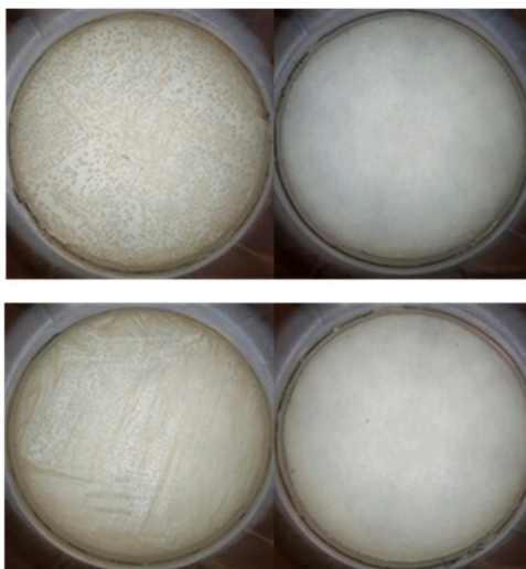
Figure 5. Photos of the petri dishes containing E. coli (upper photos) and S. aureus (lower photos) cultures. The petri dishes on the left have been exposed to uncoated QCM-D crystals, while those on the right have been exposed to (Naf/Lys) 6 coated discs, under otherwise identical conditions.
