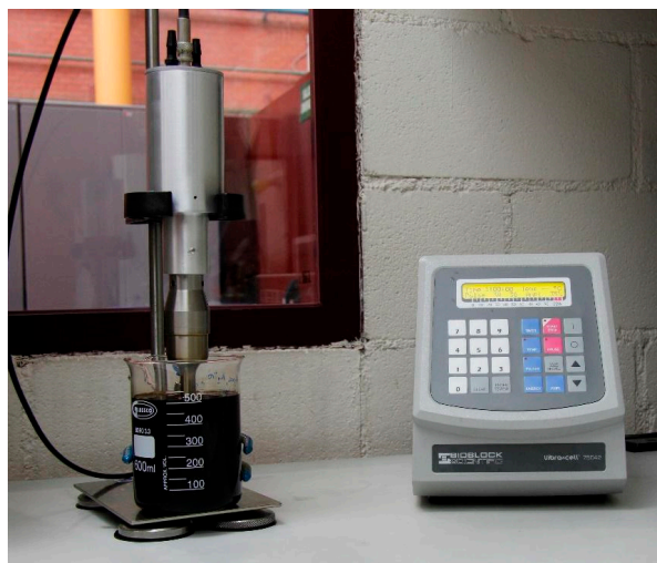
Figure 3. Sonicator 750 W used to produce the DNF.
