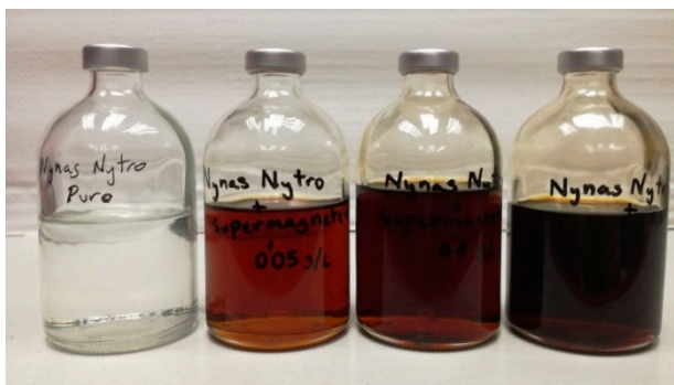
Figure 4. Samples of MO-based DNF with different concentrations of NP. From left to right: MO without NP, MO + FF2 (0.05 g/L), MO + FF2 (0.1 g/L) and MO + FF2 (0.2 g/L).
