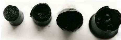
**Figure S1.** Photograph of various hydrogels from top view. Hydrogels from left to right are 3DG, GQDs/3DG-10, -40 and -80, respectively.
