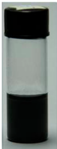
Figure S6. Dispersion of GO-TRIS-PEEP in methanol with a concentration of about 0.5 mg/mL.
