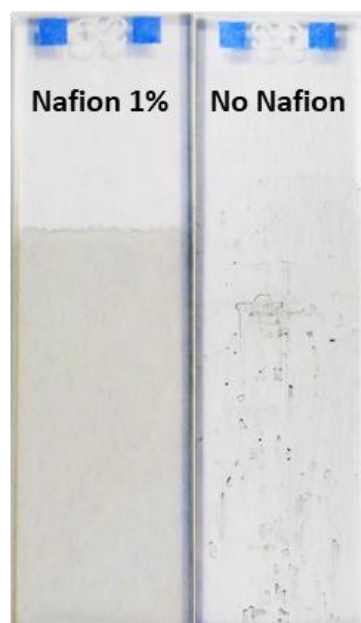
Figure S3. Optical image of Nafion/GNPs LbL films (left) and pristine GNP LbL films (right).
