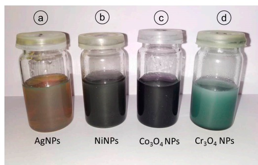
Figure 2. Pictures of synthesized colloidal samples showing the colors of final stage of solutions in each case. Different colors depict different composition of NPs.
