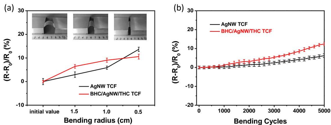
**Figure S4.** (a) Relative resistance changes of the bare AgNW TCF and the BHC/AgNW/THC TCF as a function of bending radius. (b) Relative resistance changes of the films under bending tests with 5000 bending cycles under bending radius of 1 cm. The relative change in resistance is expressed as  $(R-R_0)/R_0$ , where R is the resistance after bending tests and  $R_0$  is the resistance before bending.
