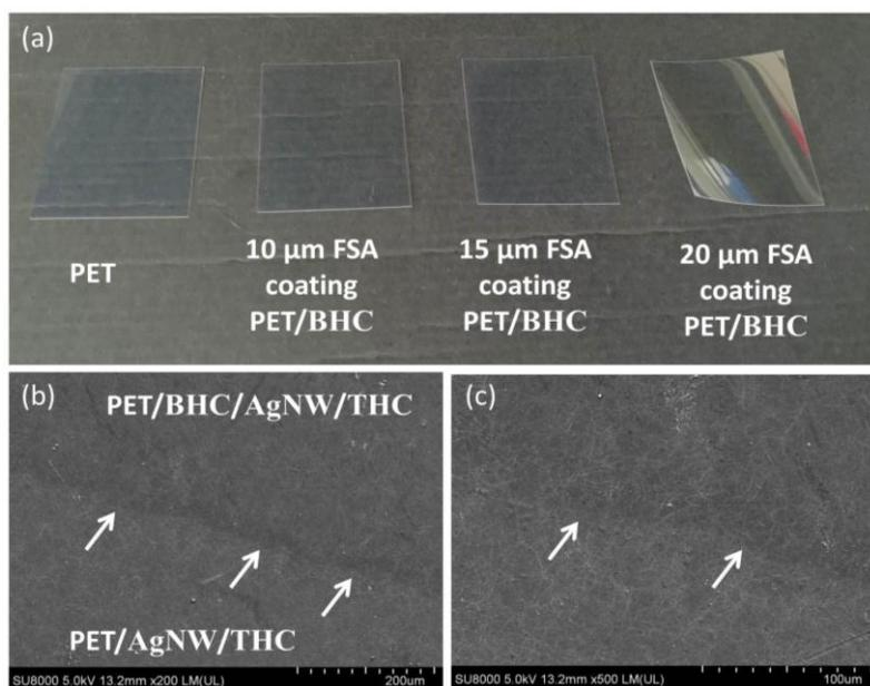
**Figure S3.** (a) The picture of PET/BHC substrates with 10 μm, 15 μm and 20 μm coating thickness. (b) Normal and (c) enlarged interface SEM image manifesting the intact AgNW film structure.
