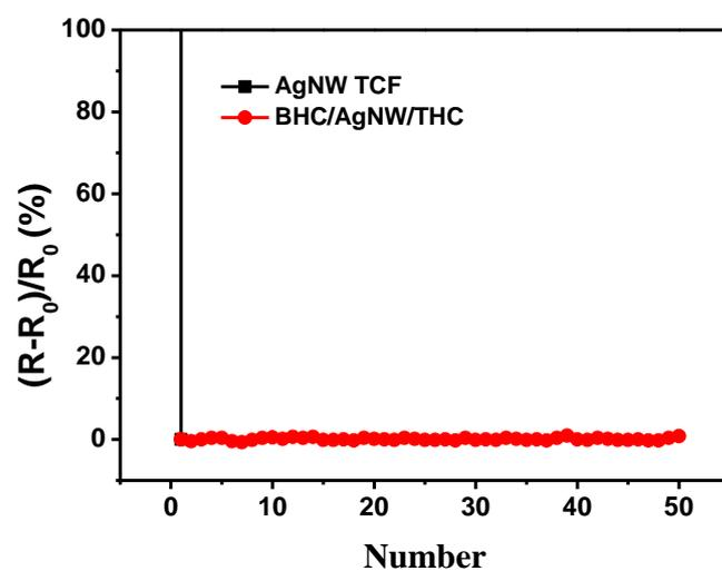
**Figure S2.** Relative changes in the resistance after the 3M taping test, once for the bare AgNW TCF and 50 times for the BHC/AgNW/THC TCF.
