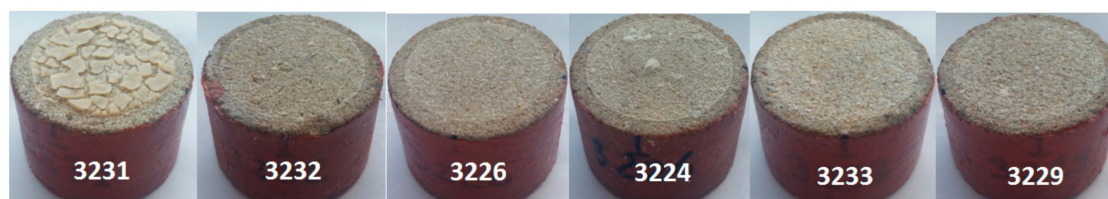
Figure 5. The cores surface after damage with S.F.
