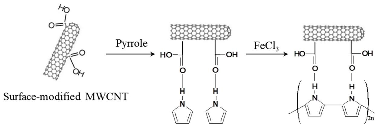
**Figure S1.** Schematic description of the synthesis of MWCNT-polypyrrole core-shell nanowire.
