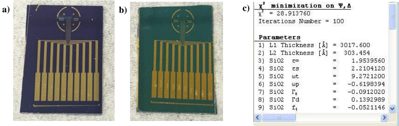
Figure S5. Optical image of the sensor (a) before and (b) after \text{Al}_2\text{O}_3 deposition (c) L1: \text{SiO}_2 and L2: \text{Al}_2\text{O}_3 thickness measured by ellipsometer.
