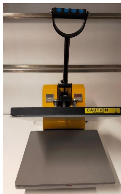
Figure S1. Image of the transfer press used for soaking of the wax barrier into the glass microfiber to define the microfluidic structure.
