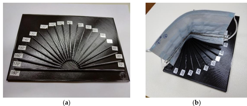
Figure 18. (a) Three-dimensionally printed component for facemask bending tests; (b) facemask placed in holder with a 90-degree bending angle.
