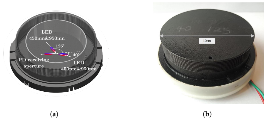
Figure 4. The design of the prototype sensor. (a) The 3D model of sensor. (b) The prototype sensor.
