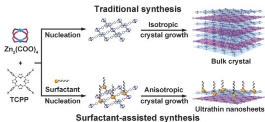
Figure 7. Scheme depicting the surfactant-mediated synthesis of 2D MOFs. The traditional synthesis method yields bulk crystals due to isotropic growth. The incorporation of the surfactant on the MOF surface results in anisotropic growth, thereby producing ultrathin nanosheets. Reproduced from [47]. Copyright 2015 Wiley Materials.
