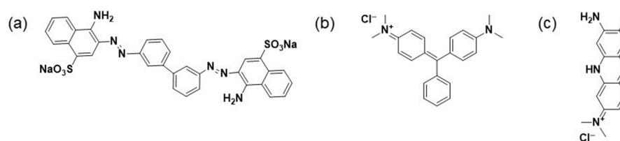
Figure 1. Chemical structures of organic dyes. (a) congo red, (b) malachite green, (c) neutral red.
