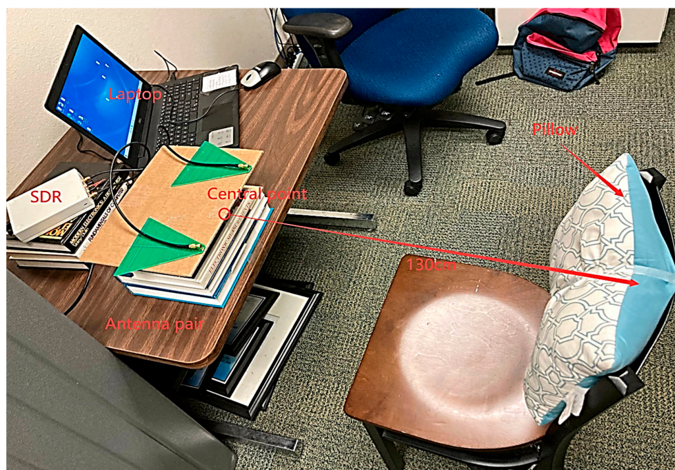
Figure 8. An example of the clinical trial setup of our NCVS system in a room of the TTUHSC Physicians Clinic.
