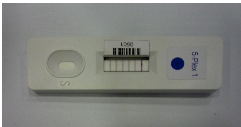
Figure 3. A commercial lateral flow test for contemporary assay of biological warfare agents.
