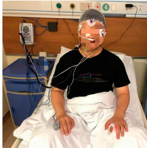
**Figure 12.** The subject with the smart ring being placed on the right index finger and the professional PSG equipment being placed on the left little finger.
