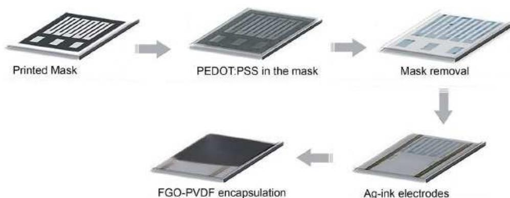
**Figure 4.** Schematic diagram of the fabrication steps of FGO–PVDF-encapsulated PEDOT: PSS thermistors [79]. Proving the robustness of a PEDOT:PSS-based thermistor via functionalized graphene oxide–poly (vinylidene fluoride) composite encapsulation for food logistics.
