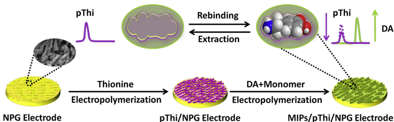
Figure 6. Schematic diagram of the MIP-based ratiometric electrochemical sensor for DA recognition. In the presence of DA in a solution, the sensor signals its presence by simultaneously decreasing the pThi- and increasing the DA-related DPV responses. Reprinted with permission from J. Yang, Y. Hu, Y. Li, Molecularly imprinted polymer-decorated signal on-off ratiometric electrochemical sensor for selective and robust dopamine detection, Biosens. Bioelectron. 135 (2019) 224–230. https://doi.org/10.1016/j.bios.2019.03.054 . Copyright 2023 Elsevier [113].
