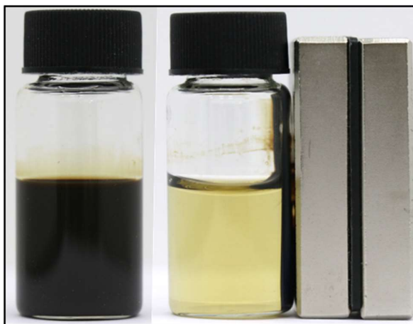
Figure S1. Magnetic adsorption diagram of magnetic nanoparticles in an aqueous solution.
