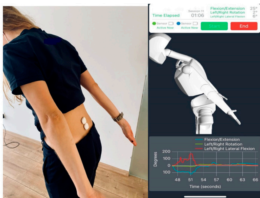
Figure 7. Application of wearable sensors in the lumbar spine. Reproducing software and recorded kinematic data. Reproduced with permission from [59] (Copyright 2022, MDPI).
