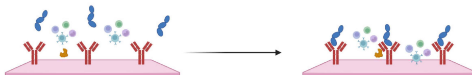
Figure 5. Schematic representation of IL-6 binding to an antibody, causing a change in system impedance.
