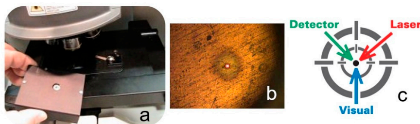
Figure 2. The alignment and calibration tool: (a) The tool to be placed on the microscope stage; (b) The bright pinhole in the optical focus centered in the binocular cross-hair; (c) A schematic diagram showing the optimal alignment of the sampling point, laser excitation, and visual spot.
