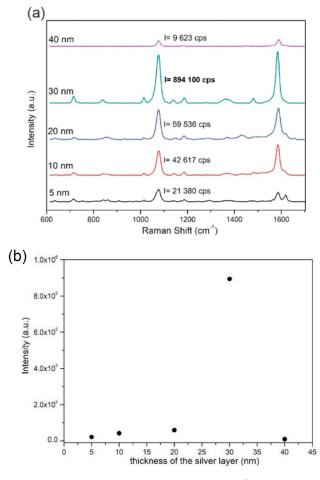
**Figure 5.** SERS spectra of *para*-mercaptobenzoic acid (p-MBA) ( $10^{-6}$  M) on PET/ITO/Ag platforms with various silver thicknesses. (**a**) Intensity of a band at 1075 cm<sup>-1</sup> in relation to sputtered silver thickness. (**b**) SERS spectra were recorded using a 785 nm laser excitation (the laser power was below 5 mW) with three accumulations for four seconds.
