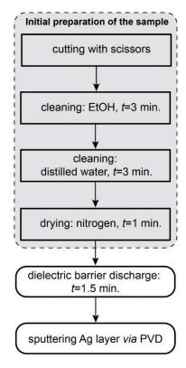
**Figure 1.** Preparation of the surface-enhanced Raman spectroscopy (SERS) platform consists of three main steps: initial preparation of the sample (cutting, cleaning and drying), modification of the surface layer with dielectric barrier discharge, and finally, sputtering a thin layer of metal with the physical vapor deposition (PVD) method.
