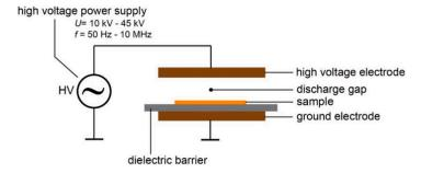
**Figure 2.** General scheme of the dielectric barrier discharge (DBD) method. The setup consists of two electrodes, the dielectric barrier on or near the one electrode, and the sample between the electrodes. The electrodes are connected to a high voltage power supply, which operates with the voltage between 10 kV and 45 kV and with the frequency between 50 Hz and 10 MHz.
