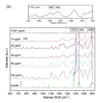
**Figure 6.** The averaged selected SERS spectra of Thiram (a) and Carbaryl (b) pesticides, measured in five different places of PET/ITO/Ag platforms. The Raman spectra of pesticides powder are presented on the bottom of each figures. The main Raman bands are indicated by dashed lines. Three accumulation for four seconds of SERS spectra were recorded using a 785 nm laser excitation (the laser power was below 5 mW).
