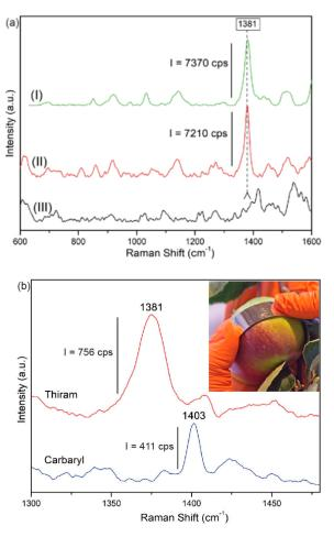
**Figure 8.** (a) SERS spectra on PET/ITO/Ag platform recorded for Thiram pesticide solution (I), Thiram in apple juice (II), and apple juice (III), and (b) the detected traces of both Thiram and Carbaryl taken from an apple's skin. The inset presents photo of pesticide collection from an apple's skin. SERS spectra were recorded using a 785 nm laser excitation with the laser power below 5 mW with three accumulations for four seconds.
