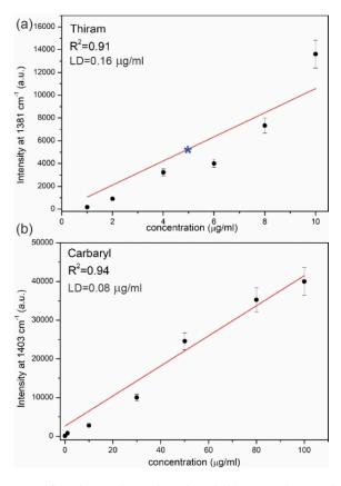
**Figure 7.** Calibration curves for Thiram (a) and Carbaryl (b) pesticides. Each point is based on the average SERS spectra taken in five different places on the PET/ITO/Ag platform. The error bars indicates 9% deviation at a chosen band. Star corresponds to the intensity of the 1381 cm $^{-1}$  band in the SERS spectrum of the apple juice with Thiram pesticide. The limit of detection (LD) for Thiram is 0.16  $\mu$ g/mL, whereas for Carbaryl it is 0.08  $\mu$ g/mL.
